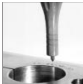
Stylus marking provides permanent identification.
